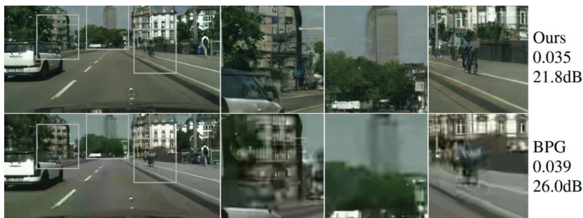
Figure 6: Figure 6 (cited from [2]): Visual comparison of images produced by a DNN-based scheme (ours) in [2] and the standard codec H.265 (BPG). BPG (Better Portable Graphics) is essentially the still image codec of H.265. The reconstructed image of the DNN-based codec (ours) is sharper and has more realistic texture but it has a lower PSNR (MSE) value.
